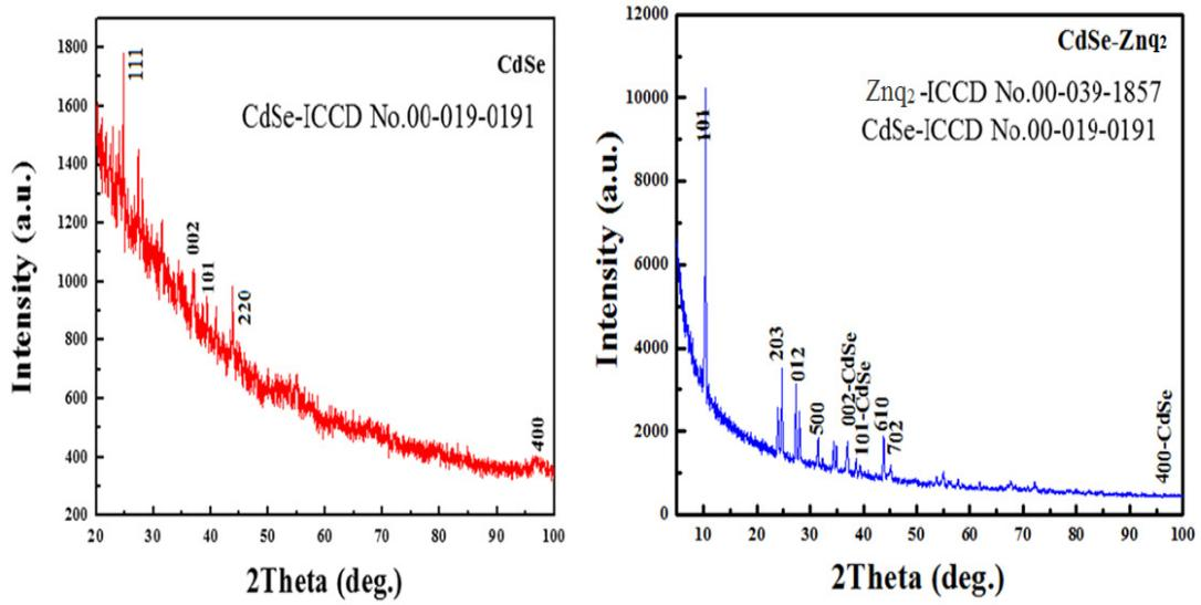
Fig. 2. XRD patterns of CdSe and CdSe-Znq<sub>2</sub>
