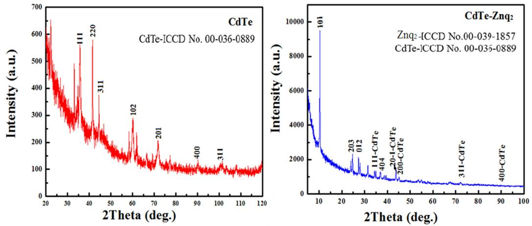
Fig. 3. XRD patterns of CdTe and CdTe-Znq<sub>2</sub>
