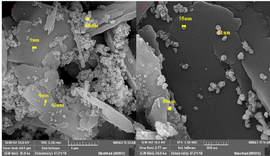
Fig. 5. SEM images of CdTe-Znq<sub>2</sub> (1) with MAG:30Kx, and (2) MAG:50Kx
