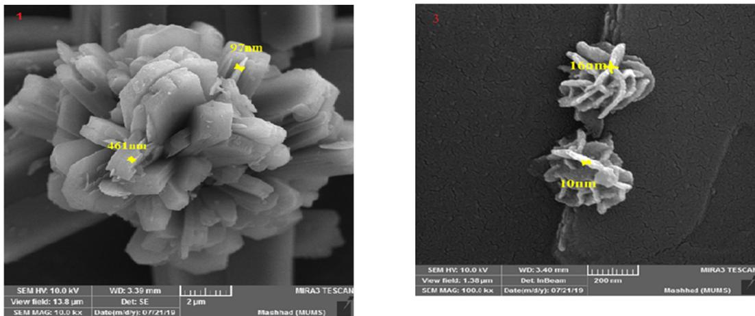
Fig. 4. SEM images of CdSe-Znq<sub>2</sub> (1) MAG:10Kx, (2) MAG: 100Kx
