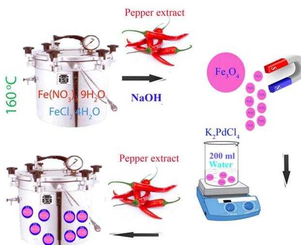
Fig. 1. Schematic of nanocomposite preparation.
