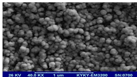
Fig. 5. SEM image of 2% Al doped ZnO thin film.
