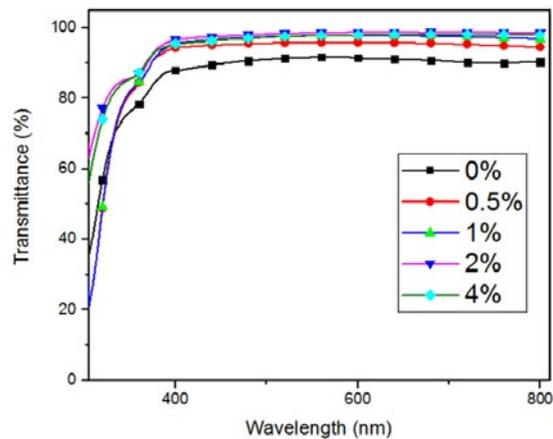
Fig. 2. UV/vis transmittance of 0 – 4 % Al doped ZnO thin films.
