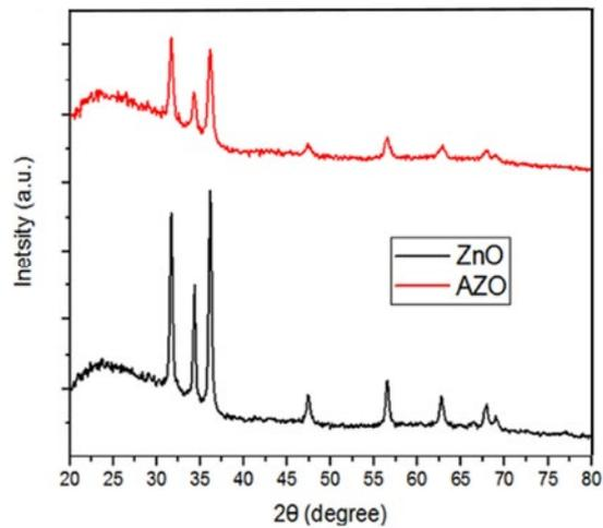
Fig. 1. XRD pattern of pure ZnO and AZO.
