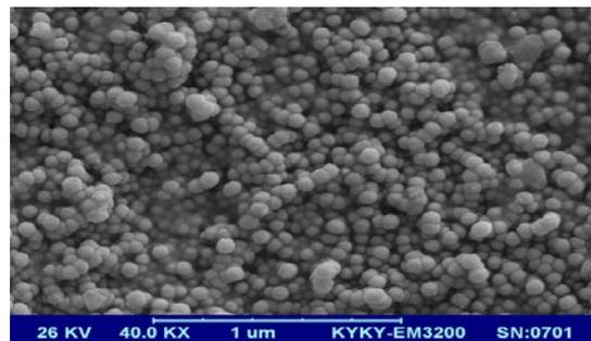
Fig. 4. SEM image of pure ZnO thin film.
