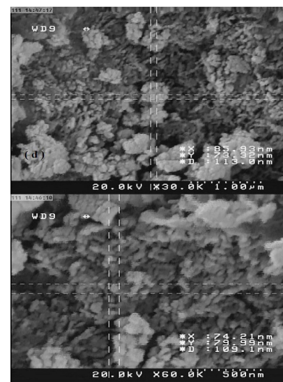
Fig. 7. SEM image of ZnS nanoparticles by thiourea and \text{Na}_2\text{S}
