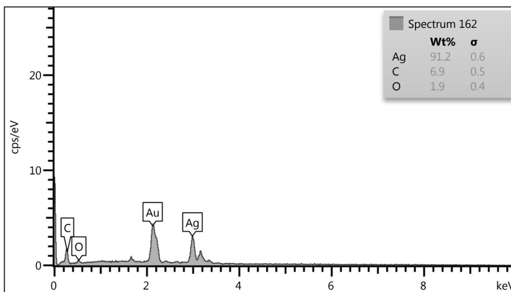
Fig. 12. Energy-dispersive X-ray (EDX ) spectroscopy of synthesized silver oxide nanoparticles (Ag<sub>2</sub>O-NPs).
