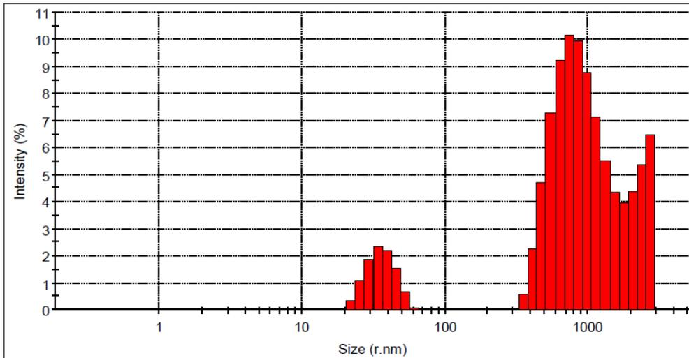
Fig. 13. DLS analysis of silver oxide nanoparticles (Ag<sub>2</sub>O-NPs).
