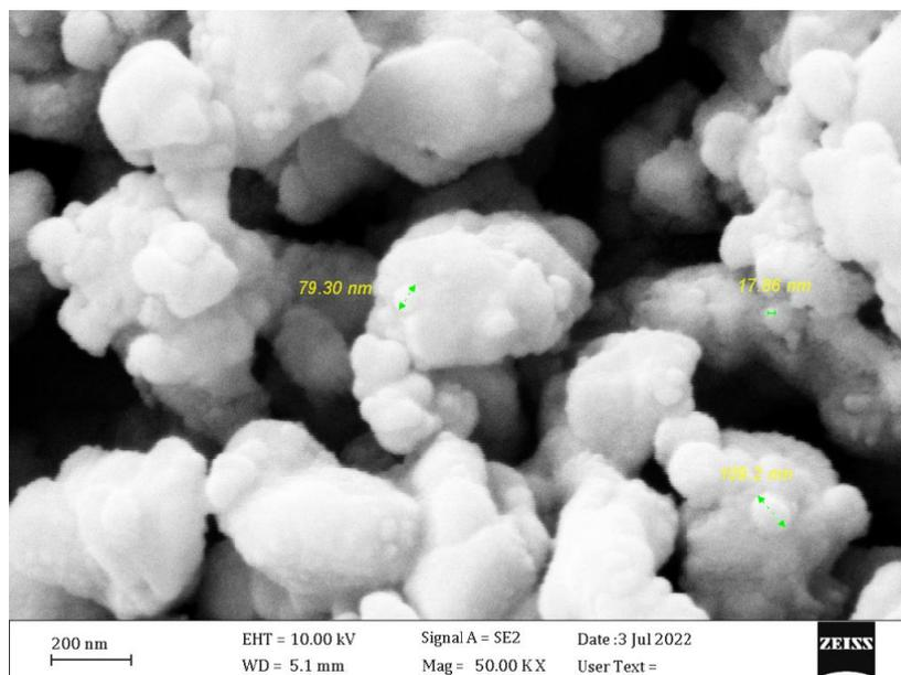
Fig. 15. FE-SEM image of Ag<sub>2</sub>O/P<sub>2</sub> matrix.
