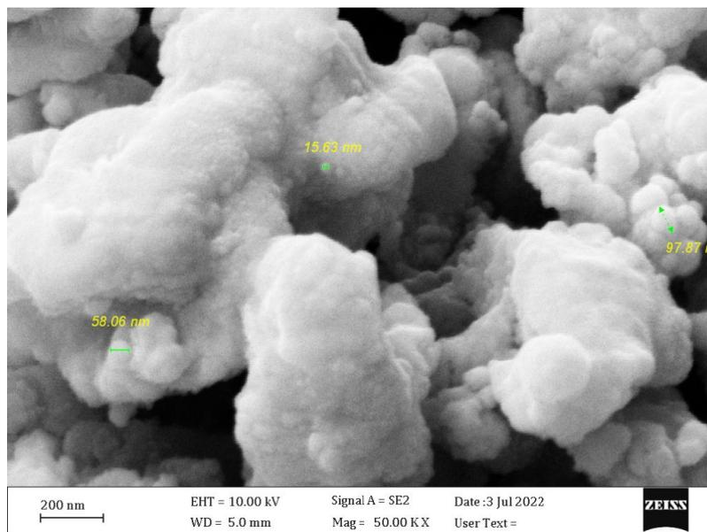
Fig. 14. FE-SEM image of Ag<sub>2</sub>O/P<sub>1</sub> matrix.
