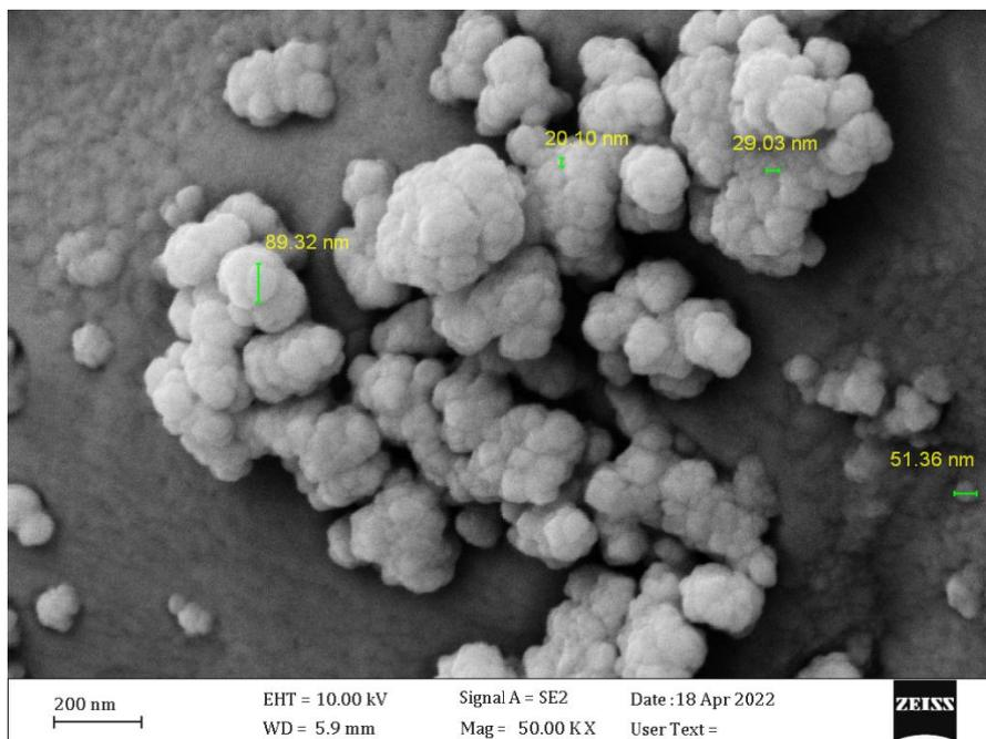
Fig. 11. FE-SEM image of silver oxide nanoparticles (Ag<sub>2</sub>O-NPs).
