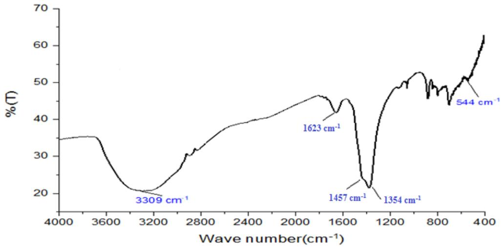
Fig. 9. FT-IR analysis of silver oxide nanoparticles (Ag<sub>2</sub>O-NPs).
