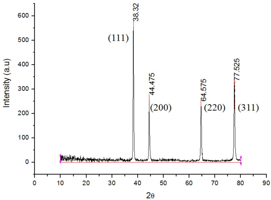
Fig. 10. X-ray diffraction pattern of silver oxide nanoparticles (Ag<sub>2</sub>O NPs).
