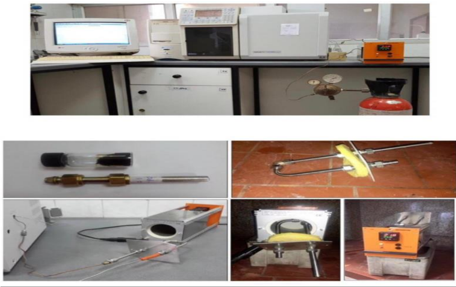
Fig. 3. Experimental setup and reactor for acetylene and ethylene selectivity.
