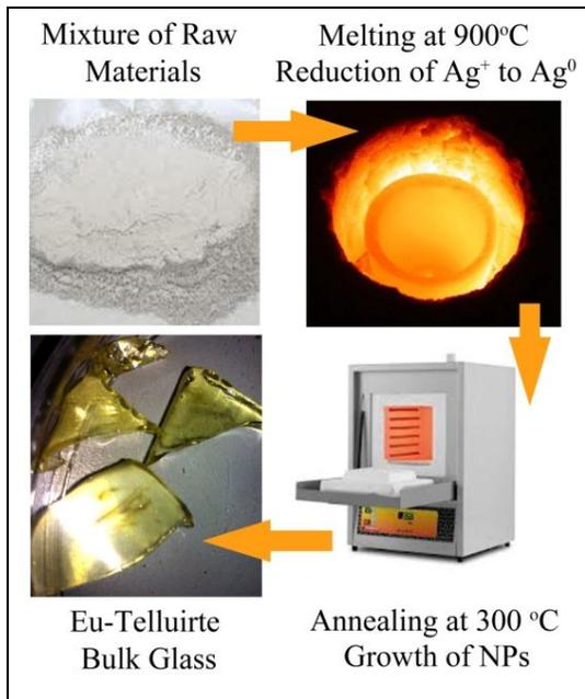
**Fig. 1.** Schematic steps of the glass preparation by the melt-quenching technique.
