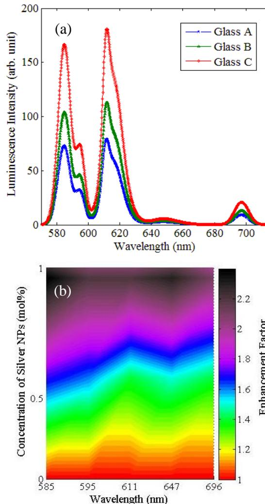
**Fig. 4.** (a) Photoluminescence spectrum of the  $\text{Eu}^{3+}$ -doped tellurite glass with (B,C) and without (D) silver NPs. (b) Enhancement factor as a function of emission wavelength and concentration of the silver NPs.
