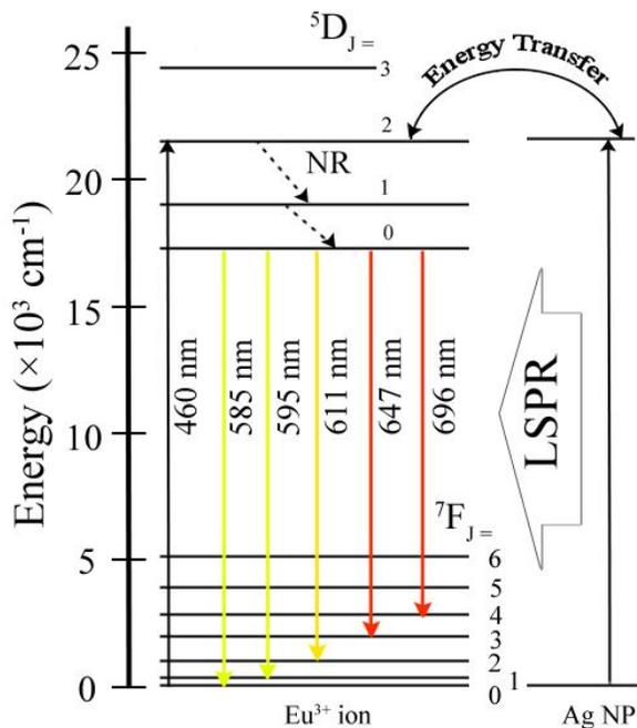
**Fig. 5.** Schematic partial energy level diagram of the  $\text{Eu}^{3+}$  ion in vicinity of a silver NP doped tellurite glass.
