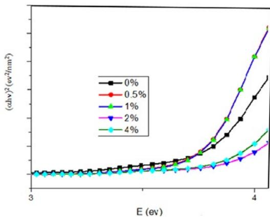
Fig. 3. Optical band gap of 0-4 % Al doped ZnO thin films.
