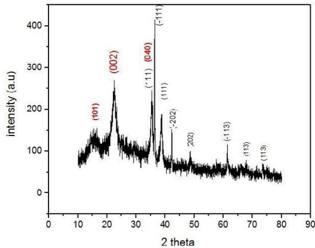
Fig. 3. XRD of CuO- Cellulose nano rods.
