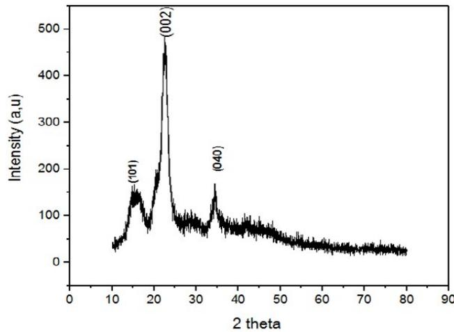
Fig. 2. XRD of pure cellulose nano rods.
