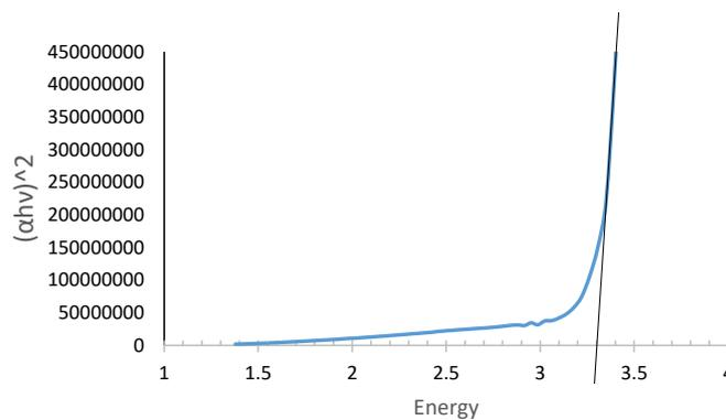
Fig. 8. Energy band gap of CuO - Cellulose nano rods
