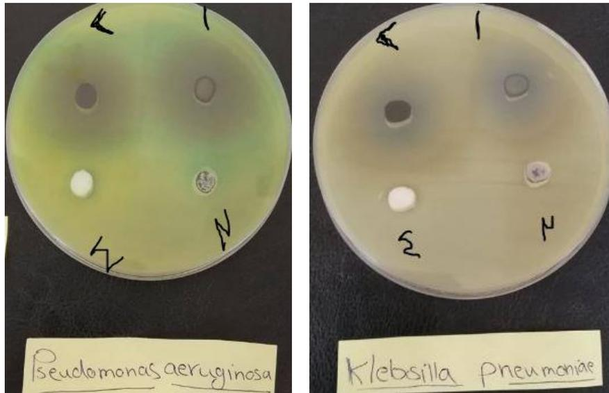
Fig. 9. Optical micrographs of agar plates, showing the variation in the zone of inhibition zone (1) CuO nano sheet (2) CuO-cellulose nano rod and (3) control (4) cellulose nanocomposite for pneumonia and pseudomonas.
