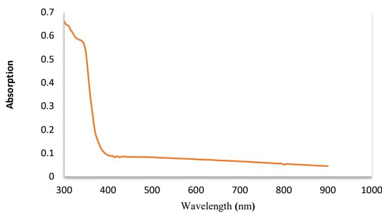
Fig. 5. UV-Vis absorption spectrum of CuO nano sheets.
