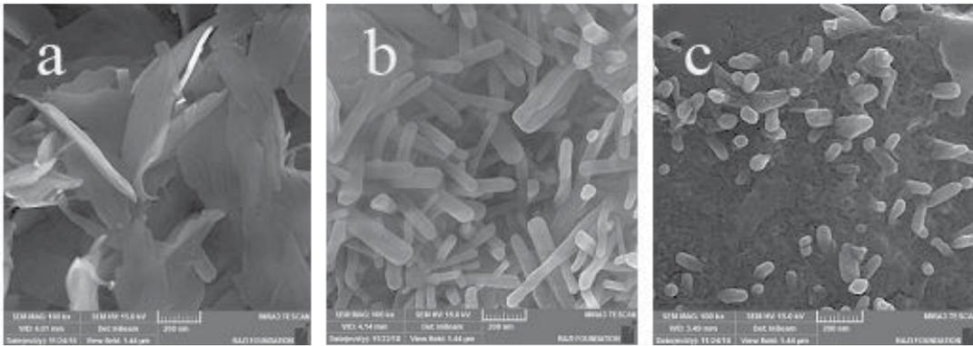
Fig. 4. FESEM images of a) pure CuO nano sheets b) pure cellulose nano rods and c) CuO – cellulose nano rods.
