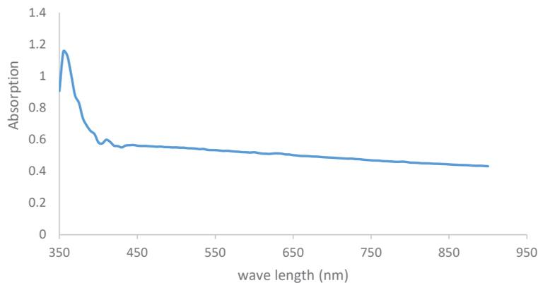
Fig. 6. UV-Vis absorption spectrum of CuO – cellulose nano rods.
