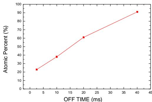
**Fig. 2.** Cu atomic percentage of NiCu nanowires arrays as a function of off-time.
