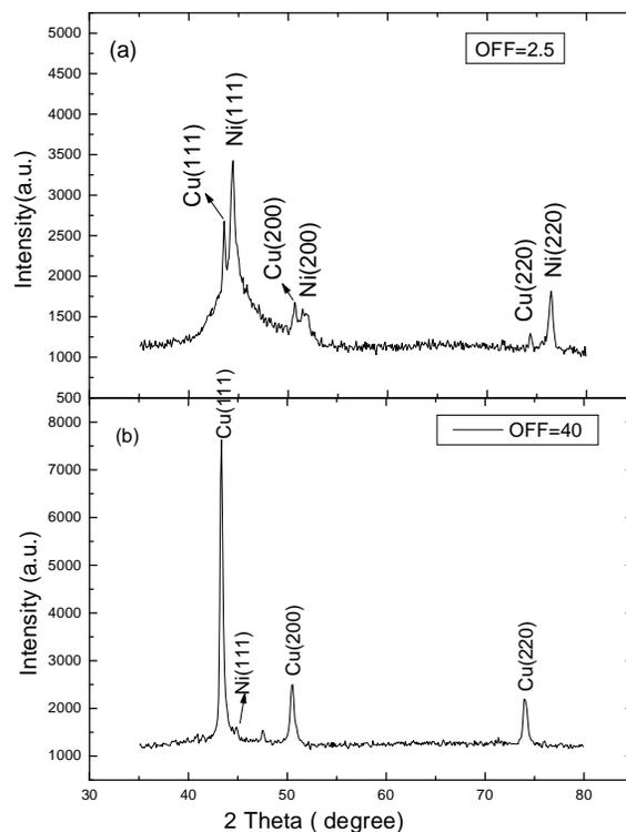
**Fig. 3.** X-ray diffraction patterns of prepared NiCu nanowires with a)2.5 ms and b)40 ms off-times.
