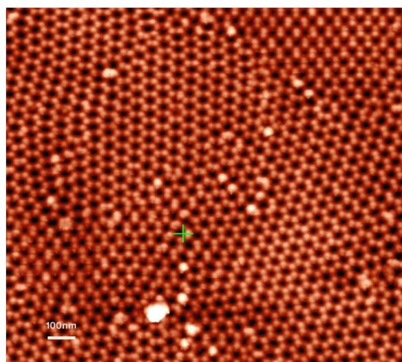
**Fig.1.** A top view AFM image of the nanopore arrays fabricated by using of the two step anodization method.
