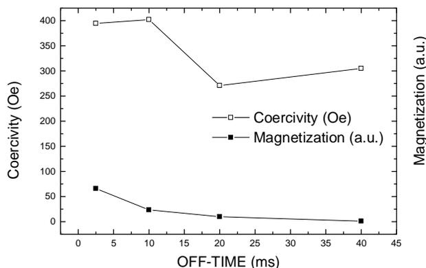
**Fig. 5.** Coercivity and magnetization of as-deposited samples as a function of off-times.
