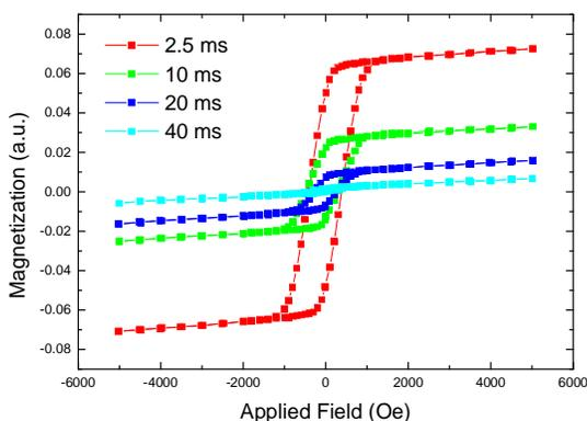
**Fig. 4.** Hysteresis loops of the as-deposited samples prepared with different off-times.
