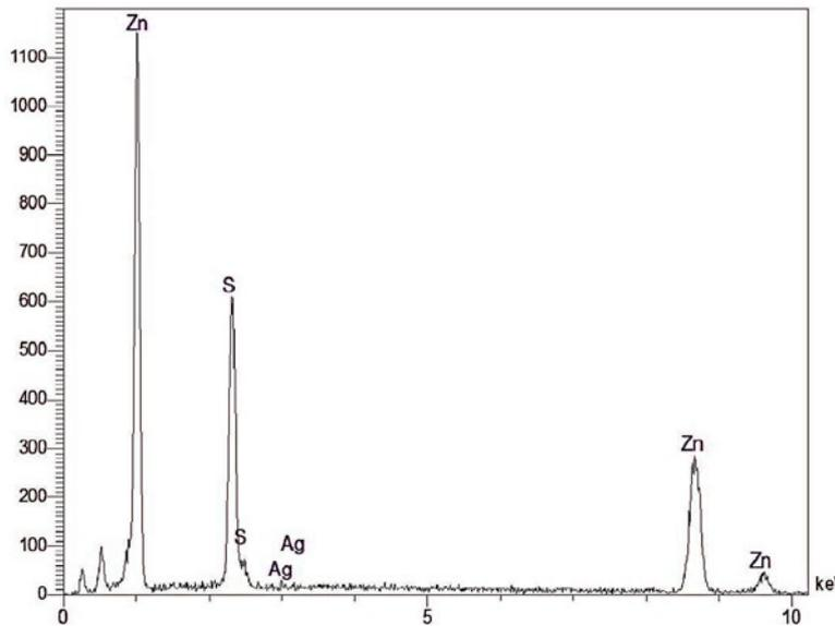
Fig. 2. The EDX spectrum of Ag-doped ZnS.
