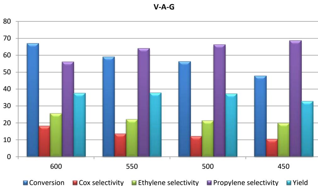
Fig. 13. Selectivity values of ethylene, propylene and carbon dioxide, propylene yields for catalysts of V-A-G at different temperatures (°C)
