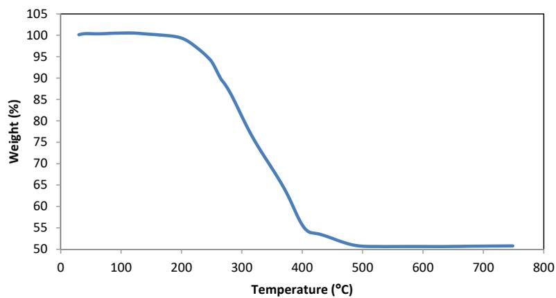
Fig. 7. TGA profiles for sample of V-ODA-G.
