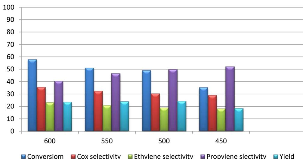
Fig. 11. Selectivity values of ethylene, propylene and carbon dioxide, propylene yields for catalysts of V-ODA-G at different temperatures (°C)
