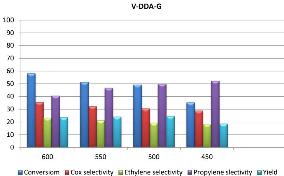
Fig. 12. Selectivity values of ethylene, propylene and carbon dioxide, and propylene yields for catalysts of V-DDA-G at different temperatures (°C)
