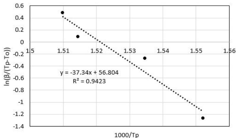
Fig. 5. Variation of  $\ln(\beta/T_p^2)$  versus  $1000/T_p$  (Kissinger plot) for different heating rates.
