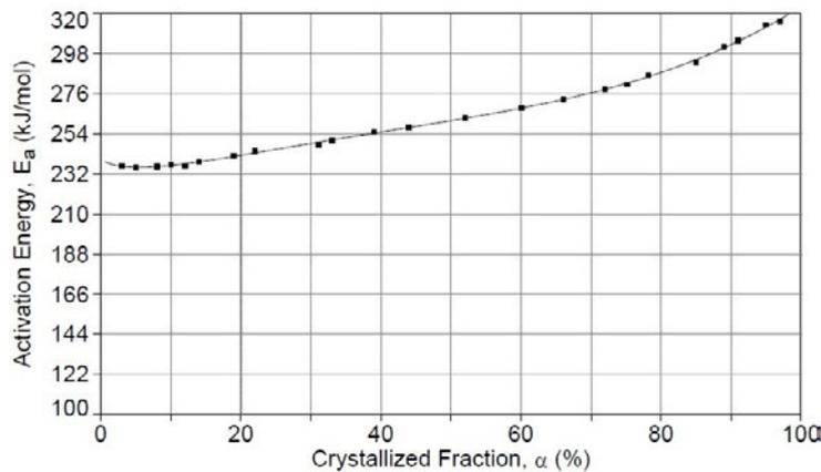
Fig. 9. Dependence of local activation energy,  $E_a(\alpha)$ , on crystallized volume fraction,  $\alpha$ , using FWO method ( $E_a = 240.4018 - 2.4088\alpha + 0.9431\alpha \ln(\alpha) - 0.0057\alpha^{2.5} + 0.00046\alpha^3$ ).
