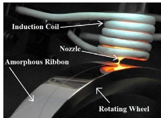
Fig. 1. Melt Spinning Process [7]
