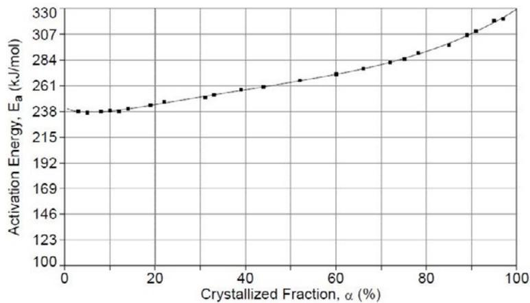
Fig. 8. Dependence of local activation energy, E<sub>a</sub>(α), on crystallized volume fraction, α, using KAS method (E<sub>a</sub>=242.3568-2.5461α+0.9922α Ln(α)-0.0059α<sup>2.5</sup>+0.00048α<sup>3</sup>).
