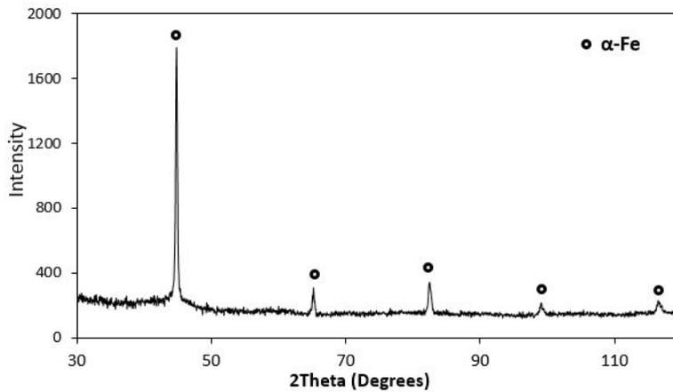
Fig. 12. XRD patterns of  $Fe_{85.3}B_{11}P_3Cu_{0.7}$  ribbons annealed at  $440^\circ C$  for 10 minutes.
