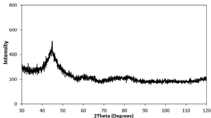
Fig. 2. X-ray diffraction pattern from the free surface of as-spun  $Fe_{85.3}B_{11}P_3Cu_{0.7}$  ribbon.
