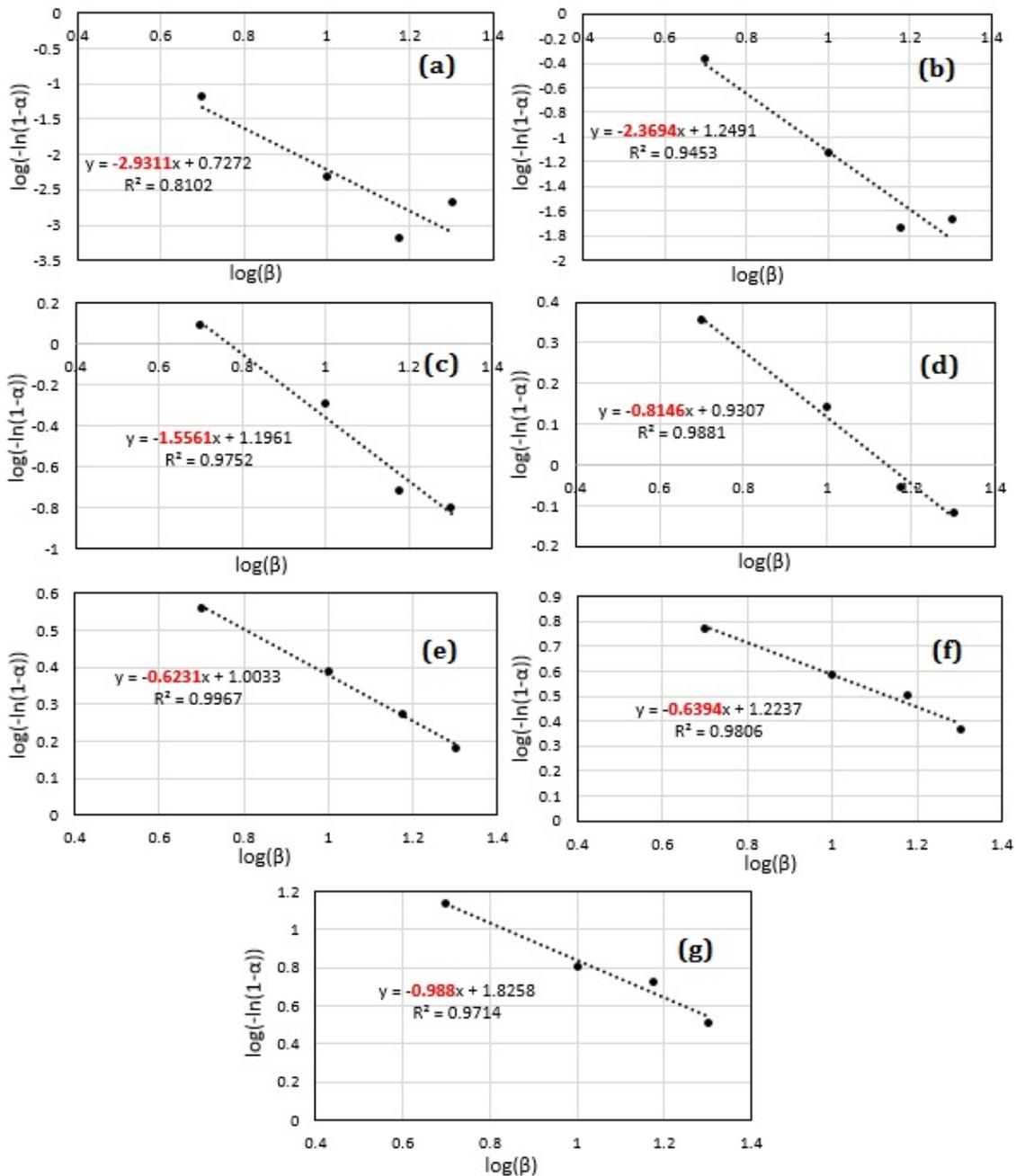
Fig. 10. Variation of Log [-Ln (1- $\alpha$ )] versus log ( $\beta$ ) for various temperatures: a) 360°C, b) 370°C, c) 380°C, d) 390°C, e) 400°C, f) 410°C, g) 420°C
