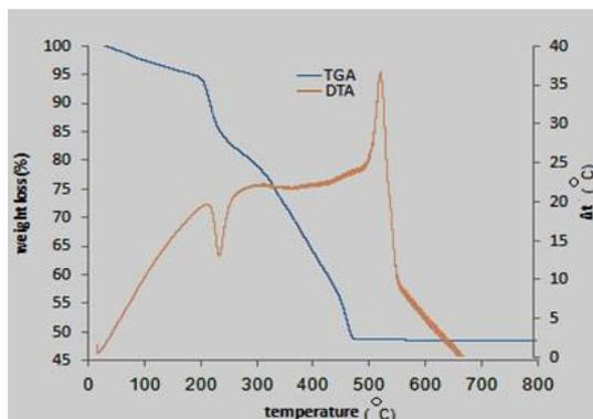
Fig. 5. Thermal behavior of compound  $[Pb(gly)_2]_n$  **1**.
