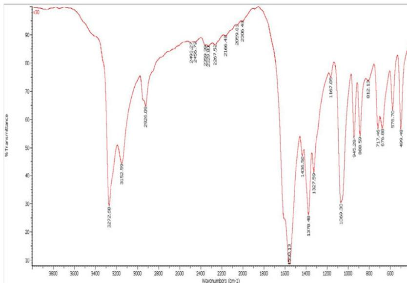
Fig. 4. IR spectra of the compound  $[Pb(gly)_2]_n$  (1).
