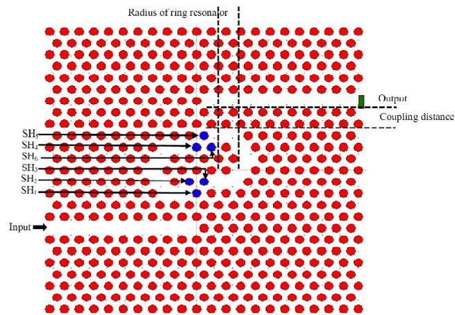
**Fig.1.** Sketch of the bio-sensor based on photonic crystal nano-ring resonator. Beneath the waveguide is the input and top of the waveguide is the output. The coupling distance, sensing holes, and the radius of ring resonator are marked on figure.
