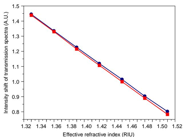
**Fig.5.** Normalized curve of the intensity of resonant wavelength with respect to the effective refractive index in sensing hole. Curves marked by closed circle and closed square represent normalized curves of SH<sub>1</sub> and SH<sub>5</sub>, respectively.
