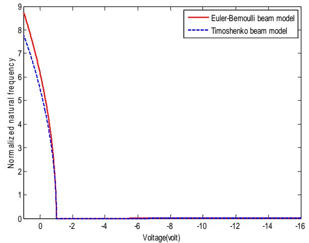
**Fig. 7.** Variation of the normalized fundamental natural frequency of Timoshenko and Euler-Bernoulli simply-supported NWs with voltage  $V$  ( $L/h = 40$ ).
