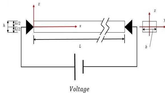
**Fig. 1.** Piezoelectric NW with rectangular cross section and its coordinate system
