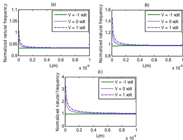
**Fig. 3.** Variation of the normalized fundamental natural frequency of Timoshenko simply-supported NW with length  $L$  for different values of voltage (a)  $L/h = 5$ ,
