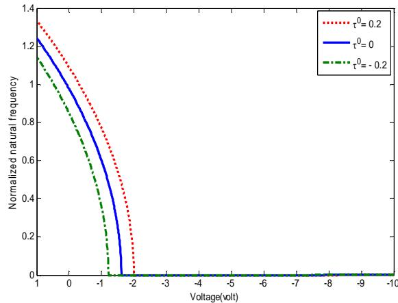
**Fig. 5.** Variation of the normalized fundamental natural frequency of Timoshenko simply-supported NW with voltage  $V$  for different values of  $\tau^0$  ( $L/h = 10$ ).
