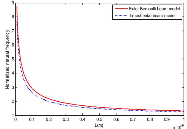
**Fig. 6.** Variation of the normalized fundamental natural frequency of Timoshenko and Euler-Bernoulli simply-supported NWs with length  $L$  ( $L/h = 40$ ).
