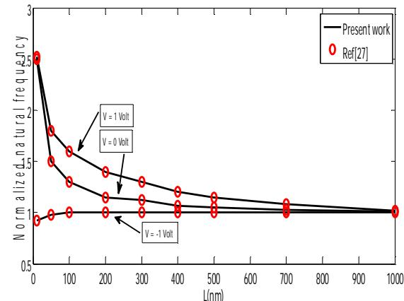
**Fig. 2.** Variation of the normalized fundamental natural frequency of Euler-Bernoulli simply-supported NW.
