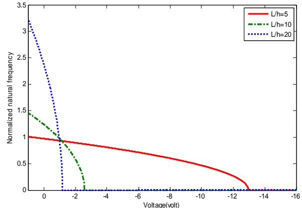
**Fig. 4.** Variation of the normalized fundamental natural frequency of Timoshenko simply-supported NW with voltage  $V$  for different values of  $L/h$ .
