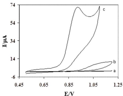
**Fig 2.** Cyclic voltammograms of (a) bare GCE in blank solution, (b) bare GCE in the presence of 2mM SMZ, (c) MWCNT-GCE in the presence of 2mM SMZ. B-R buffer (pH 6.0) solution, scan rate:  $100 \text{ mVs}^{-1}$ .
