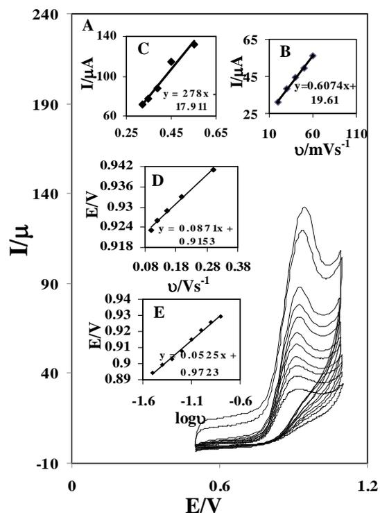
**Fig 4.** (A) Cyclic voltammetric responses of 2mM SMZ at MWCNT-GCE (B-R buffer (pH 6.0)) at scan rates, (inner to outer) 20, 30, 40, 50, 60, 80, 100, 120, 150, 200, 300  $\text{mVs}^{-1}$ . (B and C) The plots of peak currents vs scan rate and square root of scan rate, respectively. (D and E) The variation of peak potential vs  $\nu$  and  $\log \nu$ , respectively.
