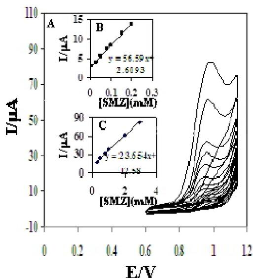
**Fig 5.** (A) Cyclic voltammograms of SMZ with various concentration in B-R buffer (0.04 M, pH 6.0) at scan rate 100  $\text{mV s}^{-1}$ . (B and C) The plots of the I vs. SMZ concentration.
