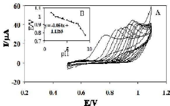
**Fig 3.** (A) Cyclic voltammograms of 2 mM SMZ at MWCNT-GCE for various pH values (from right to left) 1.5, 2.0, 2.5, 3.0, 4.0, 5.0, 6.0, 6.5, 7.0, 7.5, 8.0, 9.0 in B-R buffer, scan rate  $50 \text{ mVs}^{-1}$ . (B) plot  $E^{0'}$  vs. pH for MWCNT-GCE.
