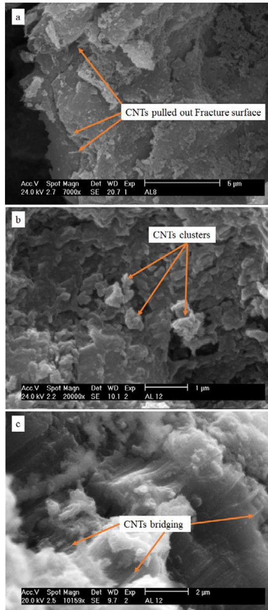
Fig. 4. (a) Fracture surface of Al-8wt. % CNTs nano-composite showing smooth surface of CNTs pulled out from the matrix and CNTs embedded in matrix (b) CNTs clusters in Al-12wt. % CNTs and (c) nanotube bridging.
