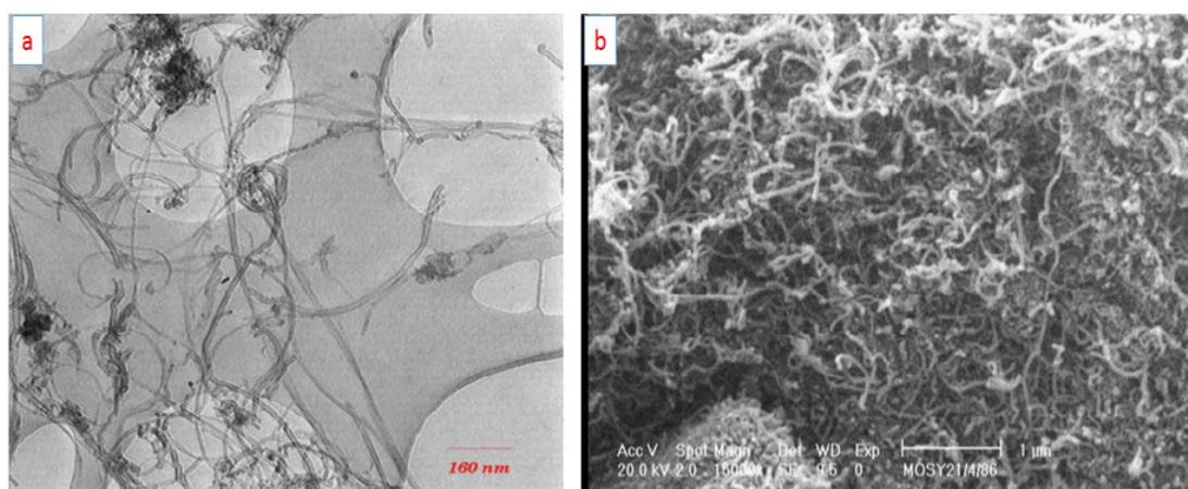
Fig. 1. TEM and SEM micrographs of MWCNTs: a- TEM and b- SEM.
