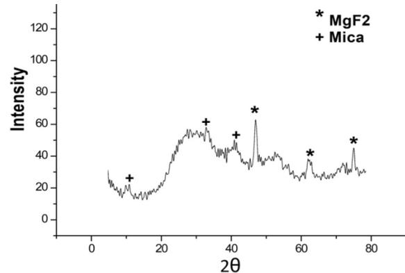
Fig. 4. XRD pattern of samples nucleated at 580 °C for 5 h.
