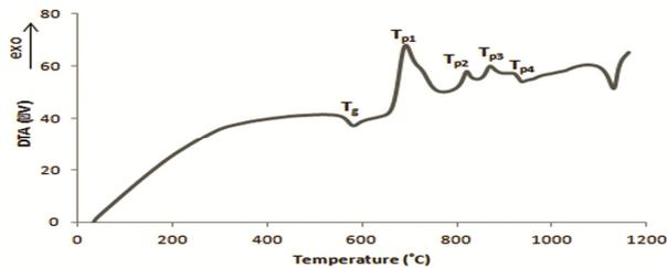
Fig. 1. DTA curve of the parent glass.
