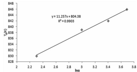
Fig. 12. Plot of  $T_g$  vs.  $\ln\alpha$  for the parent glass.
