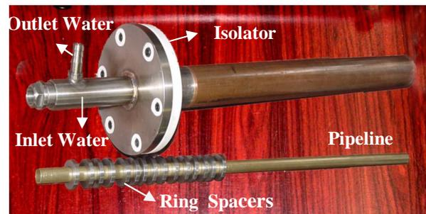
Fig. 2. Cylindrical cathode and cathode assembly.
