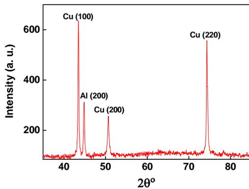
**Fig. 4.** X-ray diffraction patterns of Al/Cu multilayer film at 250 °C.
