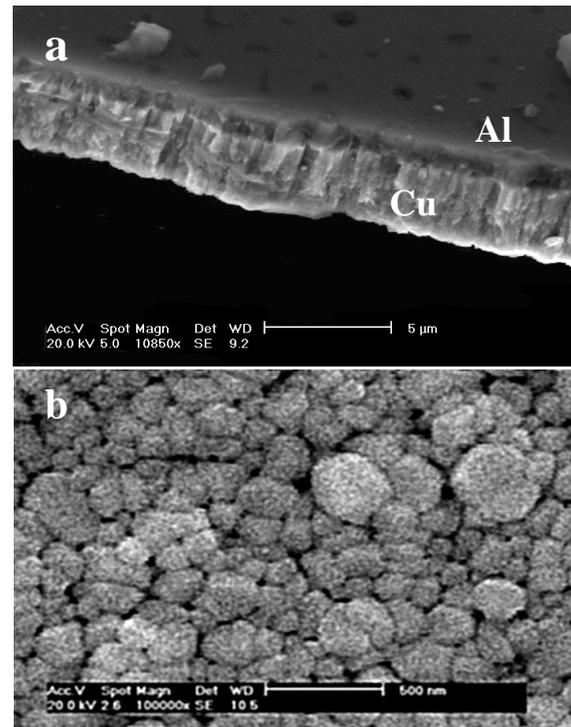
**Fig. 5.** (a) The cross sectional and (b) top view SEM micrograph of Al-Cu multilayer film.
