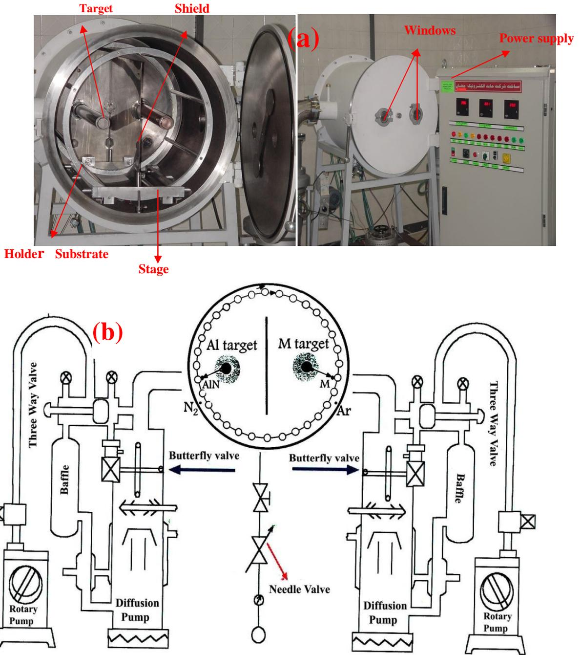
**Fig. 1.** (a) Double targets cylindrical DC magnetron sputtering system and (b) typical illustration of diagrammatic form of a cylindrical vacuum chamber and vacuum line
