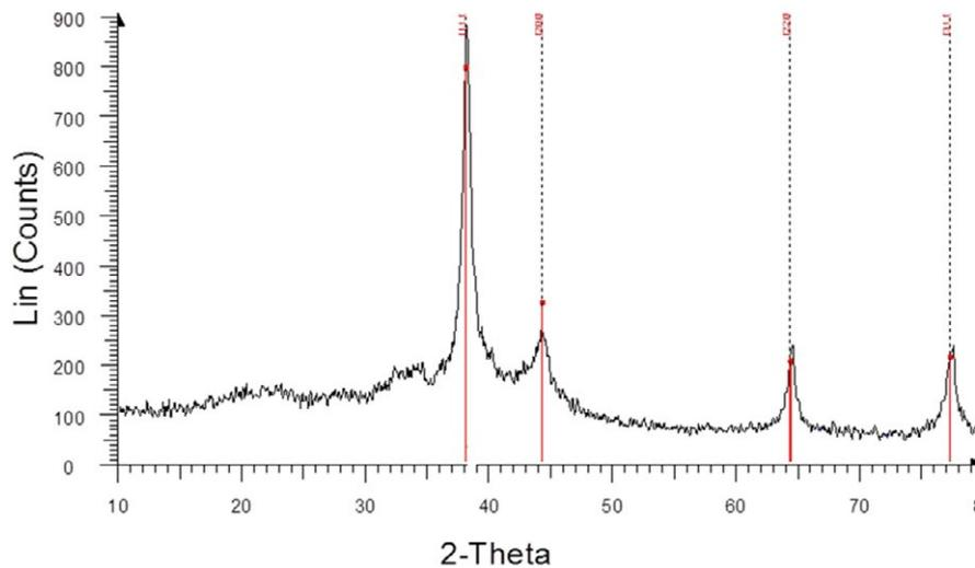
Fig. 1. XRD patterns of synthesized SNPs.
