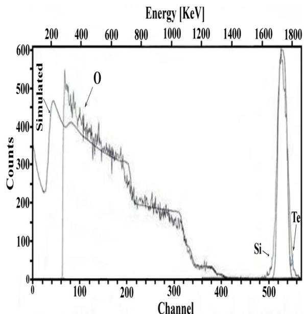
Fig. 1. Example of RBS spectrum for tellurium film.
