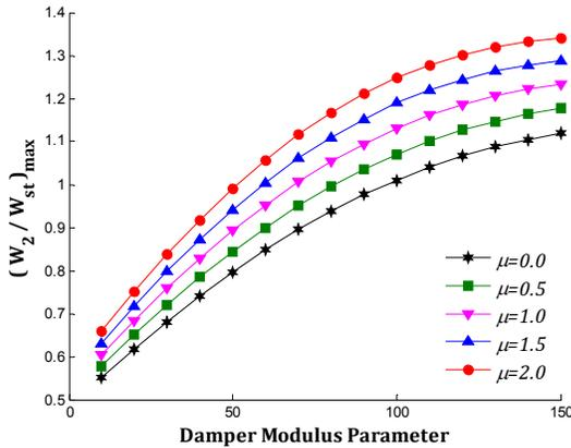
**Fig. 3.** The dimensionless displacement with respect to the damper modulus parameter for (a) SLGS-1 (b) SLGS-2
