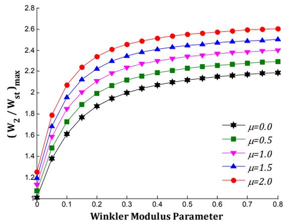
**Fig. 2.** The maximum dimensionless displacement of coupled SLGSs versus the Winkler modulus parameter (a) SLGS-1 (b) SLGS-2
