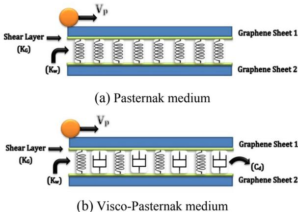
Fig.1. Coupled system of SLGSs subjected to the moving nano-particle
