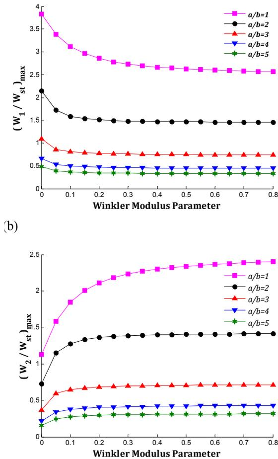
**Fig. 6.** The effect of aspect ratio ( $a/b$ ) on the maximum dynamic displacement for (a) SLGS-1 (b) SLGS-2
