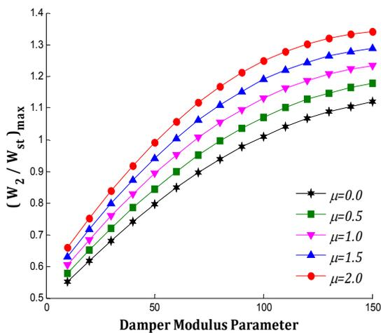
The maximum dimensionless displacement of coupled SLGSs versus the shear modulus parameter (a) SLGS-1 (b) SLGS-2
