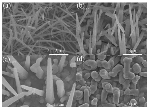
**Fig. 5.** SEM images of GeNWs with different ratio of Ar and H<sub>2</sub> as carrier gas.
