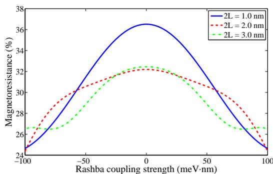
**Fig. 3.** Plot of the magnetoresistance as a function of Rashba spin-orbit coupling strength for different values of domain walls distances in the anti-parallel configuration of magnetization at the noncontacts.
