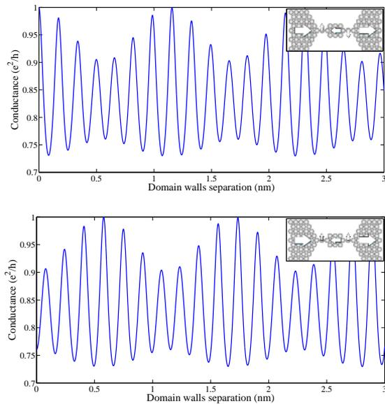
**Fig. 2.** Plot of conductance as a function of domain walls separation without considering the spin-orbit coupling effects in two parallel (lower) and anti-parallel (upper) configurations of magnetization at the noncontacts.
