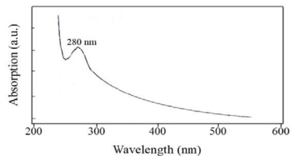
**Fig. 4.** UV-Vis diffuse reflectance spectra of  $\text{La}_{0.99}\text{VO}_4: \text{Tm}_{0.01}^{3+}$  nanosheets.
