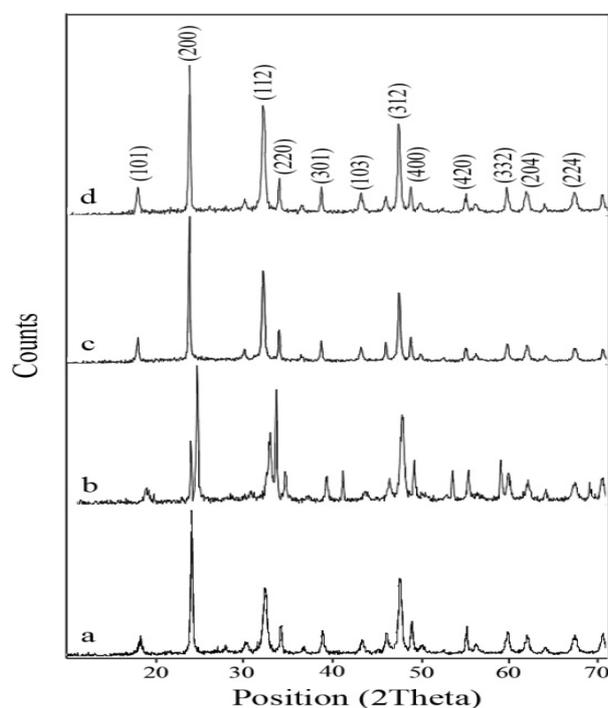
**Fig. 1.** XRD patterns of: (a)  $\text{La}_{0.99}\text{VO}_4:\text{Tm}_{0.01}^{3+}$  (b)  $\text{La}_{0.96}\text{VO}_4:\text{Tm}_{0.04}^{3+}$  (c)  $\text{La}_{0.98}\text{VO}_4:\text{Yb}_{0.02}^{3+}$  and (d)  $\text{La}_{0.8}\text{VO}_4:\text{Tm}_{0.01}^{3+}/\text{Yb}_{0.19}^{3+}$  nanocrystal.
