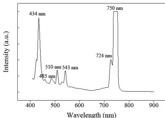
**Fig. 8.** The emission spectra of  $\text{La}_{0.8}\text{VO}_4:\text{Tm}_{0.01}^{3+}/\text{Yb}_{0.19}^{3+}$  nanocrystals.
