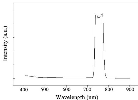
**Fig. 7.** The emission spectra of  $La_{0.98}VO_4: Yb_{0.02}^{3+}$  nanocrystals.
