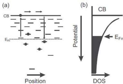
**Fig. 4.** **a)** Schematic illustration of the trap distribution and the multiple trapping–detrapping process occurring in mesoporous titania. **b)** Illustration of the density-of-states (DOS) distribution in solid films.
