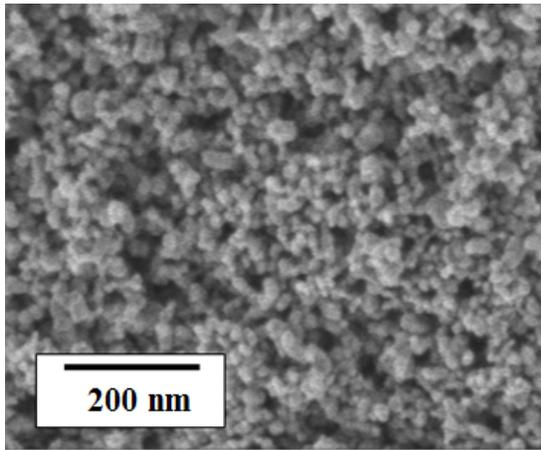
**Fig. 3.** SEM micrograph of a nanocrystalline TiO<sub>2</sub> film.
