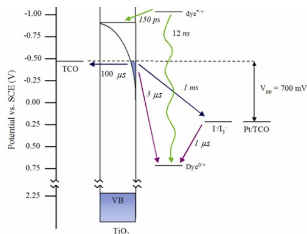
**Fig. 5.** Kinetic processes in DSSC [28].
