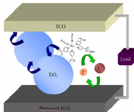
**Fig.1.** Schematic of a DSSC.
