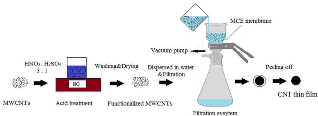
Fig. 1. Schematic of the CNT thin film fabrication process.
