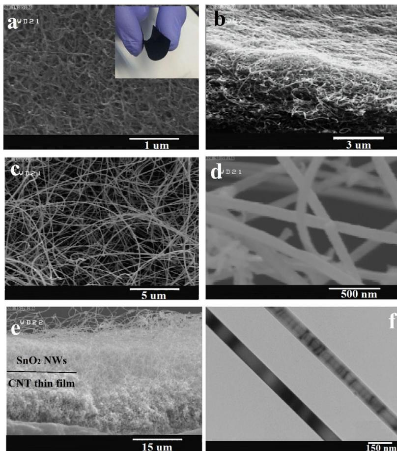
Fig. 3. SEM images of (a,b) CNT film, (c,d) SnO<sub>2</sub> on CNT film. (e) Cross-sectional SEM of SnO<sub>2</sub>/CNT film. (f) TEM image of SnO<sub>2</sub> nanowire.
