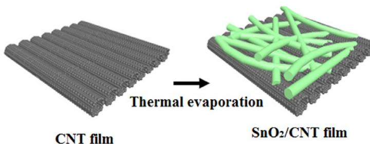
Fig. 2. Schematic diagram of SnO<sub>2</sub> NWs fabrication process on CNT film.
