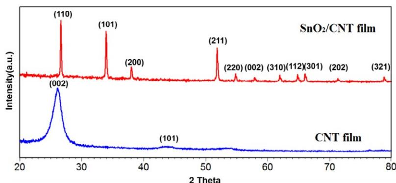
Fig. 4. XRD patterns of CNT film and SnO<sub>2</sub>/CNT film.
