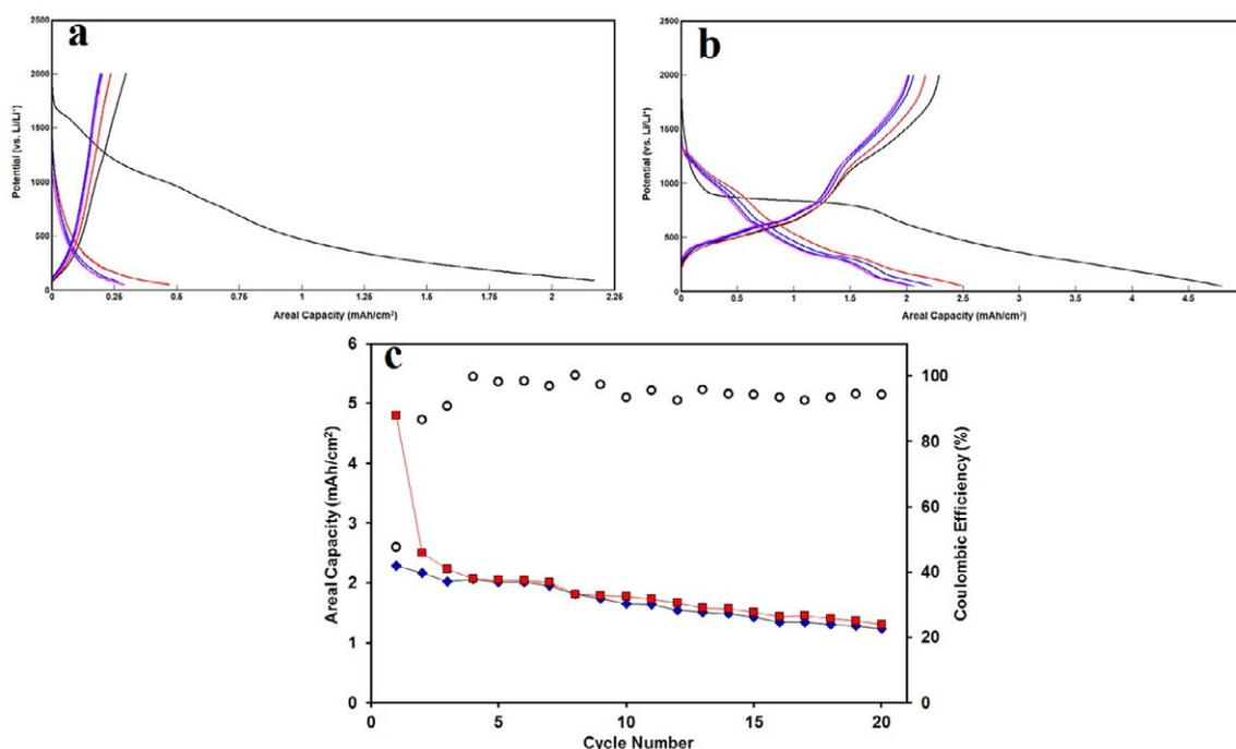
Fig. 5. Galvanostatic charge-discharge profiles of (a) CNT film, (b) SnO<sub>2</sub>/CNT film for first five cycles. (c) Cycling performance of SnO<sub>2</sub>/CNT electrode with coulombic efficiency for 20 cycles.
