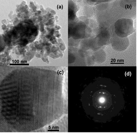
Fig. 3. TEM image of ZnO nanoparticles (a), HRTEM image of ZnO nanoparticles (c), HRTEM image of an isolated ZnO nanoparticle (c), and selected area electron diffraction (d).
