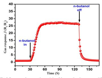
Fig. 5. Response and recovery characteristics of the sensor based on as-prepared ZnO nanoparticles at 260  $^{\rm oC}$  to 20 ppm n-butanol.
