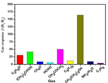
Fig. 6. Gas response of ZnO nanoparticles based gas sensors to various gases of 100 ppm at the optimal operating temperature (260  $^{\circ}$ C).
