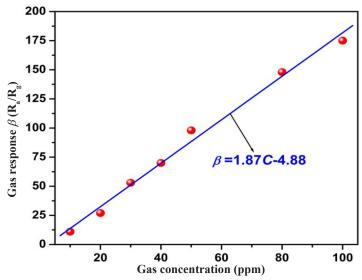
Fig. 4. Gas response of ZnO nanoparticles based gas sensors to different concentrations of n-butanol at the optimal operating temperature of 260  $^{\circ}$ C.
