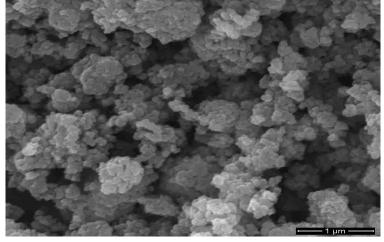
Fig. 2. SEM image of the as-prepared ZnO nanoparticles.
