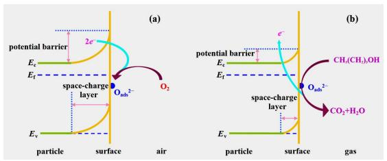
Fig. 7. A schematic diagram of the proposed reaction mechanism of ZnO nanoparticles based sensor to n-butanol.
