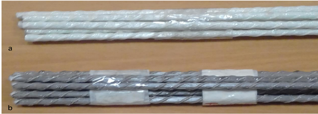
Fig. 1. The BCRs produced from thermoset resin and glass fibers: a) without MWCNTs, b) modified by MWCNTs
