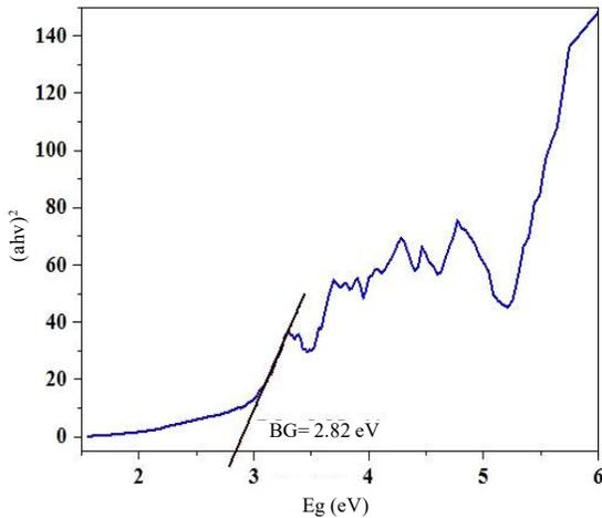
Fig. 7. The calculated band gap for 2-hydroxyacetophenone-CoFe<sub>2</sub>O<sub>4</sub>
