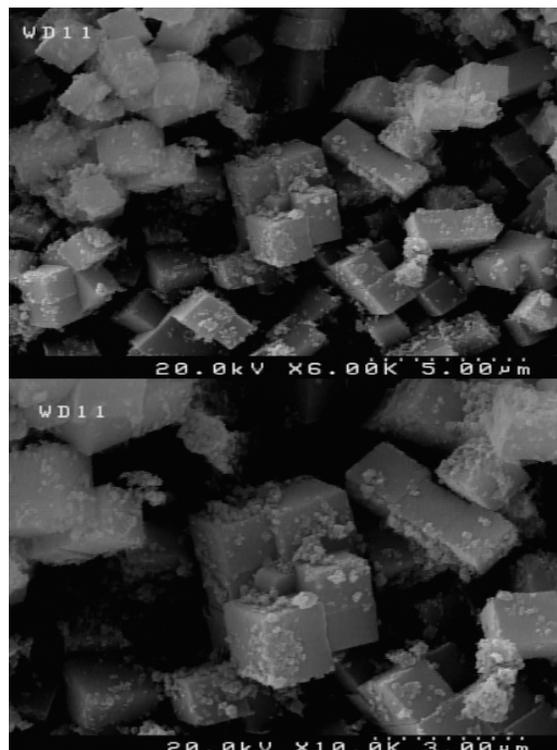
Fig. 4. SEM images of CoFe<sub>2</sub>O<sub>4</sub> stabilized by 2-hydroxyacetophenone.
