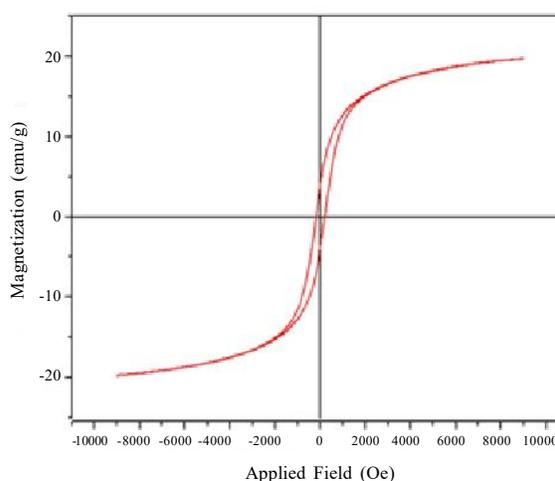
Fig. 5. Room temperature hysteresis loops of CoFe<sub>2</sub>O<sub>4</sub> nanoparticles
