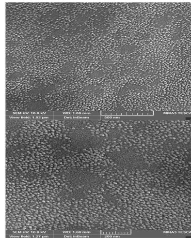
**Fig. 3.** SEM images of nanoparticles synthesized by NiNO<sub>3</sub>-PEG
