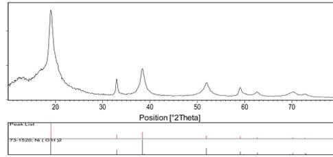
**Fig. 1.** XRD pattern of Ni(OH)<sub>2</sub> nanoparticles
