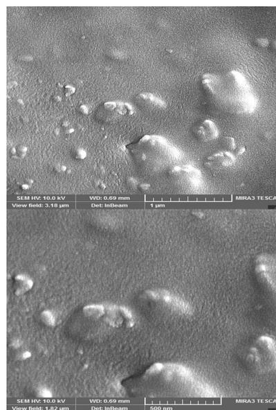
Fig. 7. SEM images of PVA-Ni(OH)<sub>2</sub> nanocomposite
