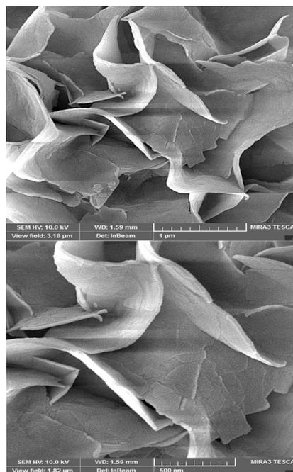
Fig. 6. SEM images synthesized by NiSO<sub>4</sub> -Triplex
