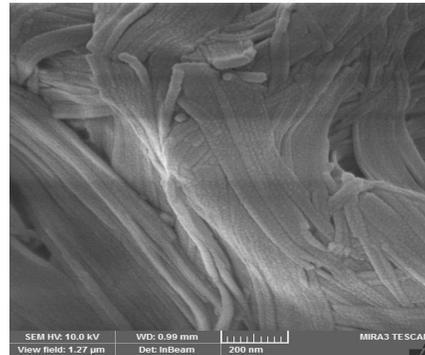
**Fig. 2.** SEM image of Ni(OH)<sub>2</sub> nanoparticles obtained by NiSO<sub>4</sub>-CTAB
