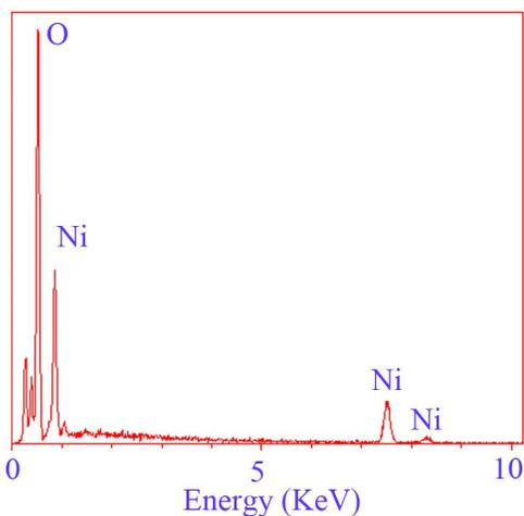
Fig. 9. EDS analysis of Ni(OH)<sub>2</sub> nanoparticles
