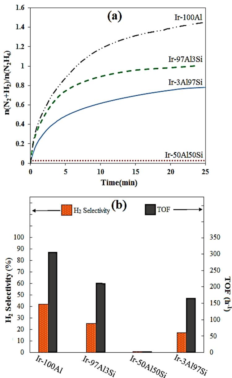
Fig. 6. (a) Time profiles, and (b) the comparison of selectivity and reaction rate for hydrous hydrazine decomposition of iridium catalysts.
