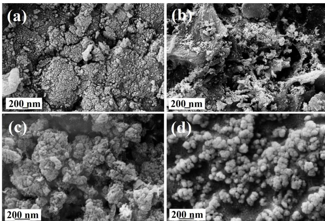
Fig. 8. FESEM micrographs of (a) Ir-100Al, (b) Ir-97Al3Si, (c) Ir-50Al50Si, and (d) Ir-3Al97Si, after decomposition of hydrous hydrazine.
