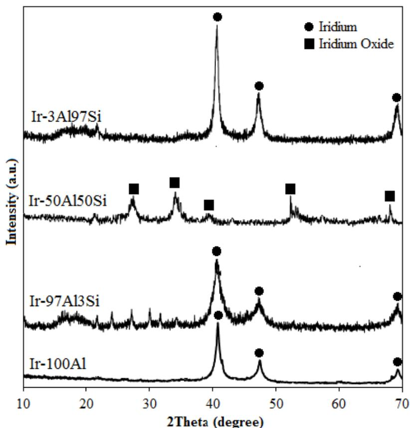
Fig. 7. XRD patterns of the iridium catalyst on different supports after decomposition of hydrous hydrazine.
