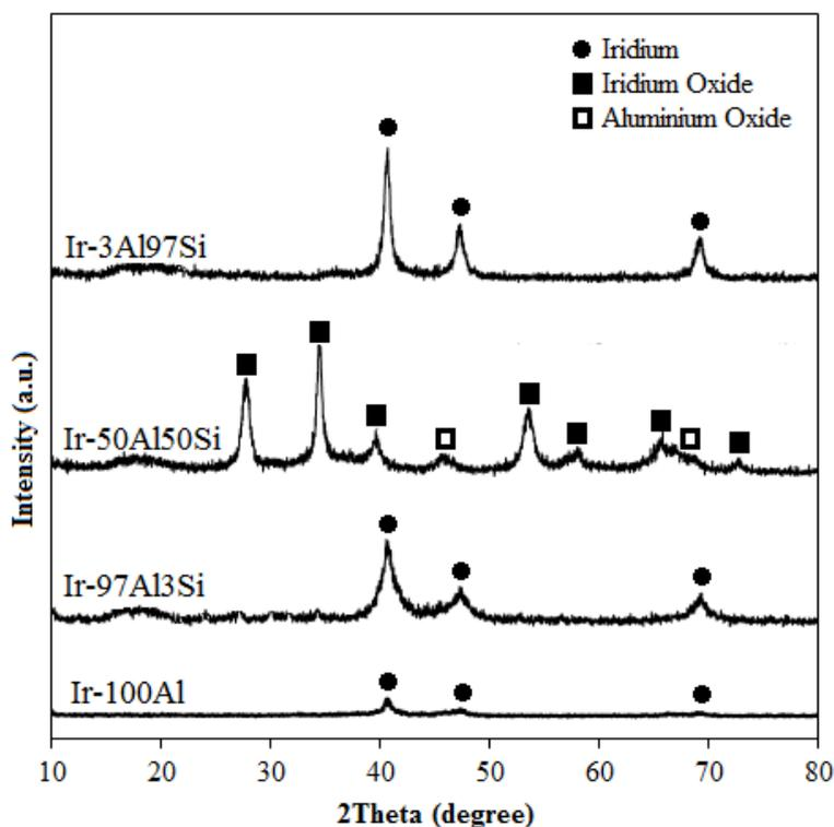
Fig. 3. XRD patterns of the iridium catalyst on different supports before decomposition of hydrous hydrazine.
