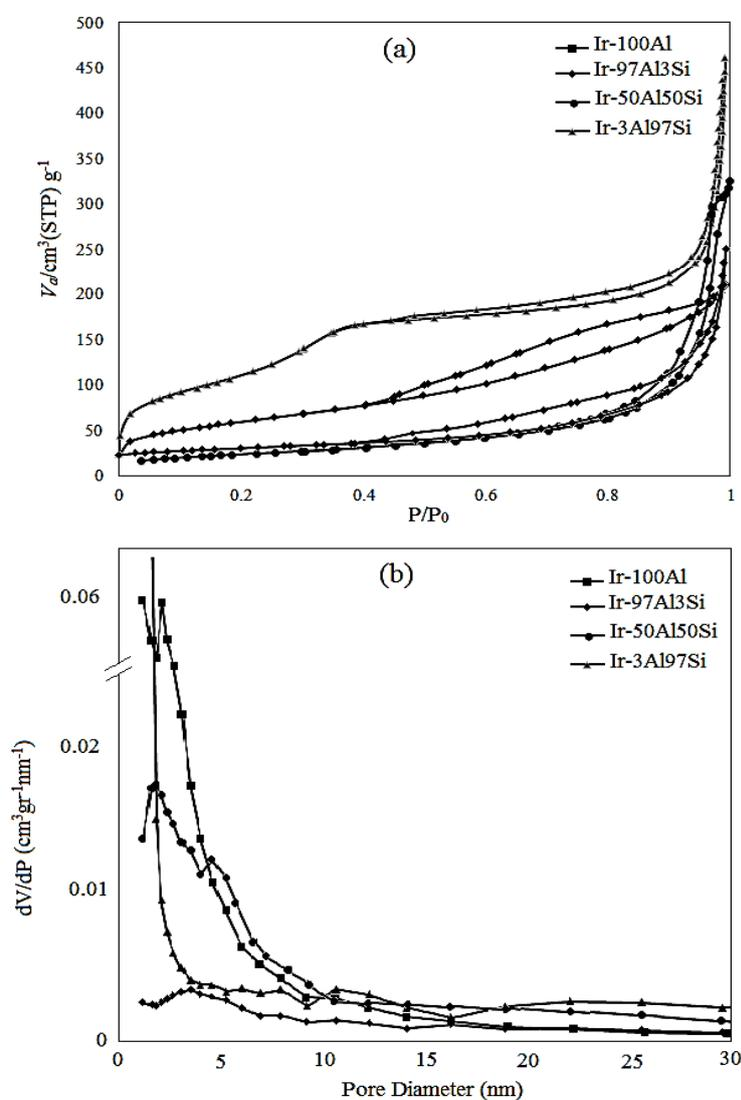
Fig. 1. (a) Nitrogen adsorption-desorption isotherms and (b) pore size distribution curves for the different catalysts.
