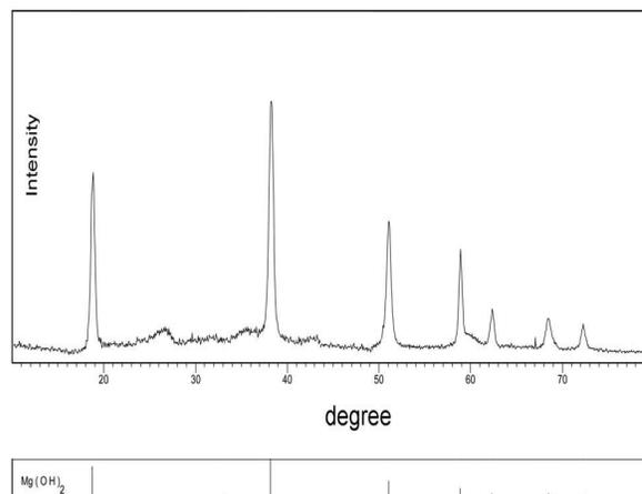
**Fig. 2.** XRD pattern of  $Mg(OH)_2$  nanoparticles
