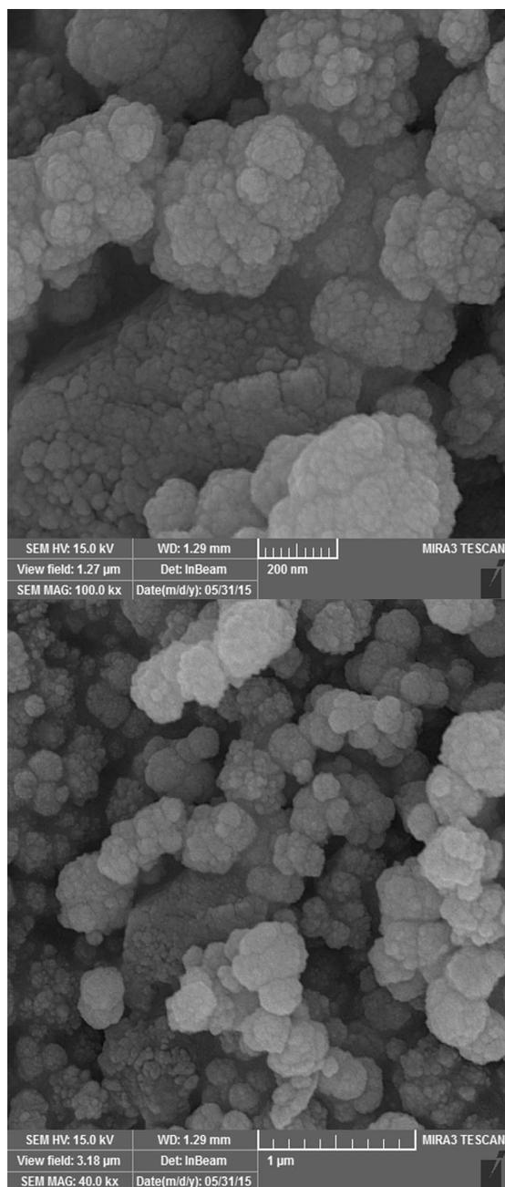
**Fig. 3.** SEM images of nanoparticles synthesized by SDS
