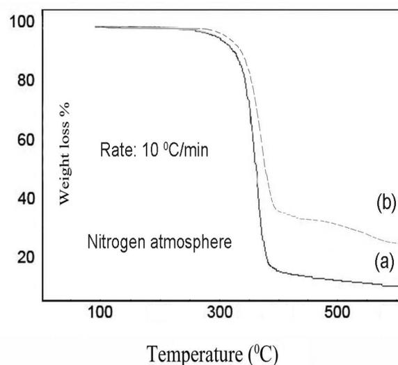
Fig. 6. TGA graphs of (a) pure CA (b) CA-MWCNT-Mg(OH)<sub>2</sub> nanocomposite
