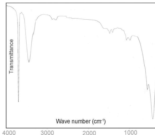
**Fig. 7.** FT-IR of Mg(OH)<sub>2</sub> nanoparticles
