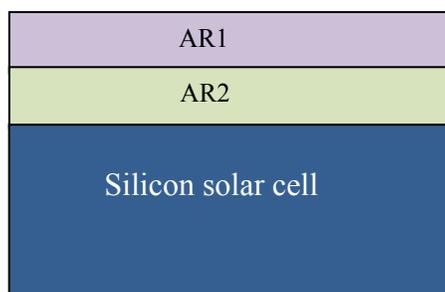
**Fig. 1.** Schematic view of DLARCs (AR1 and AR2) on the Si Solar cell.
