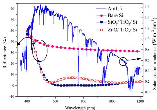
**Fig. 4.** Calculated reflection characteristics for the AR1 and the AR2 coatings as a function of wavelength and the spectral irradiance of the AM1.5.
