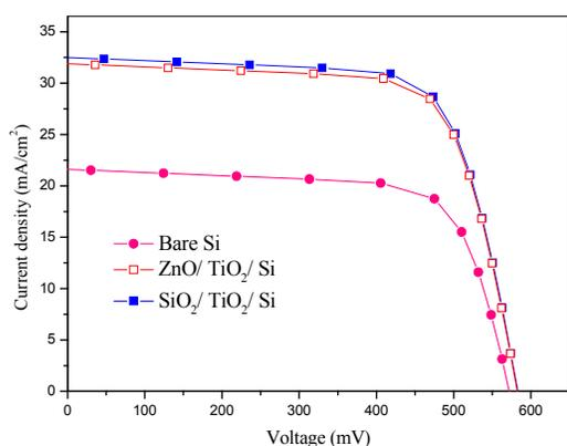
**Fig. 5.** I-V curves of the solar cell with double-layer ARCs.
