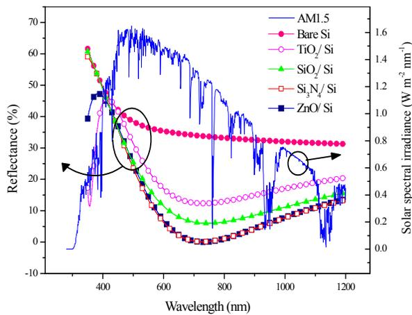
**Fig. 2.** Reflectance as a function of wavelength for the structures of Si,  $\text{TiO}_2/\text{Si}$ ,  $\text{SiO}_2/\text{Si}$ ,  $\text{Si}_3\text{N}_4/\text{Si}$ , ZnO/Si and also the spectral irradiance of the AM1.5
