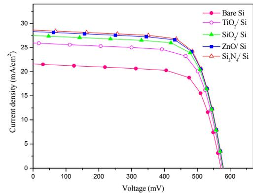
**Fig. 3.** (I–V) curves of the silicon solar cell without and with  $\text{TiO}_2$ ,  $\text{SiO}_2$ ,  $\text{Si}_3\text{N}_4$  and ZnO ARC layer.
